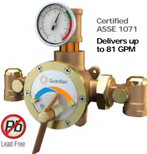
1 1/4" female pipe inlets. Inlets can be rotated 360 degrees for top or bottom supply. Each inlet has an integral water strainer, check valve & supply stop. 1 1/2" NPT female outlet.
